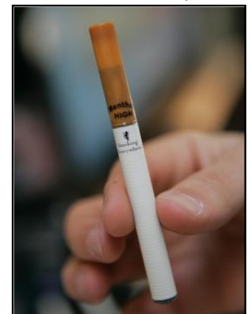
The electronic cigarette is a device that combines a computer chip, a rechargeable battery and an atomizer that emits a nicotine mist. (Jim Gensheimer/Mercury News)
